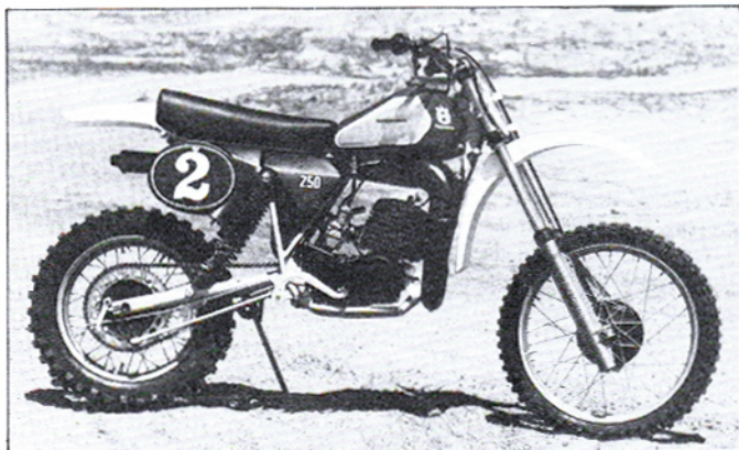
Most of the chassis components are shared on the two bikes. Long legs for sure, 12.2 inches at the rear and 11.8 inches of the finest travel around up front. Our Husky 250CR came with a special saddle that lowered the seating position one inch. It made a big difference for riders under 5'9" tall.
