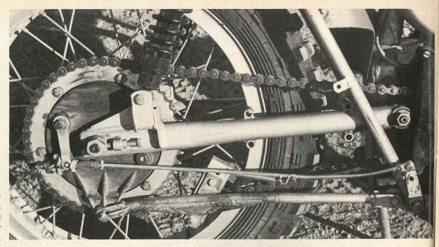
A floating rear brake is used to minimize wheel hop under hard braking.
