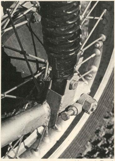
The shock mount is boxed for strength. The axle adjuster works well from the standpoint of not bending the adjusting bolt.
