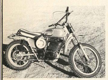
With the engine moved forward and down in the frame it's much easier to keep the front wheel on the ground under hard acceleration.
