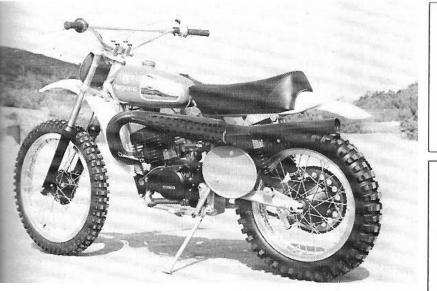
air cleaner cover, which is metal this year since the plastic units of '73 broke easily, protrudes out just far enough on the right side while the exhaust sticks out on the left. We like to grip the tank for security when things get hairy! The exhaust pipe is also new and incorporates its own built-in silencer. It really isn't as quiet as it should be but the pipe seems to be a good combination with the engine.
