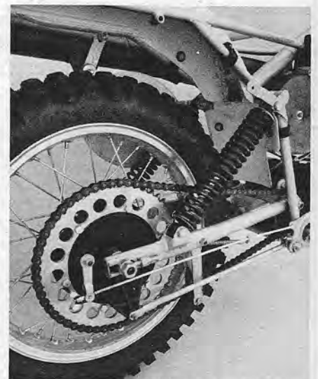
Lay-down Girling gas shocks have too-stiff springs. Lighter 117 lb/in. springs will soften ride.
