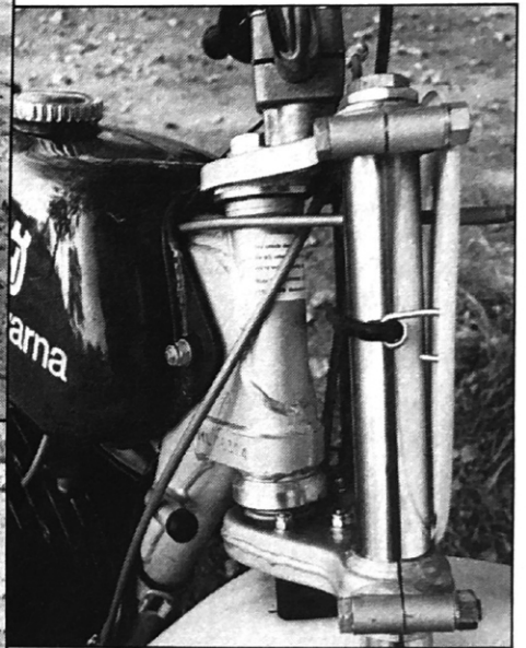
New steering head bearings live in there, and are designed to last a lot longer than previous units.
