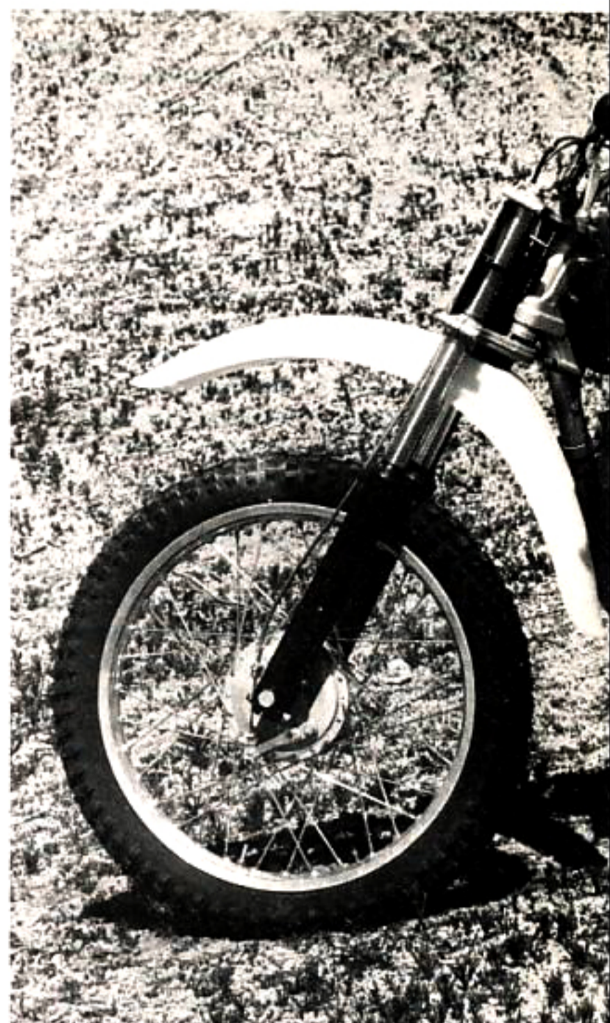
An extra inch of travel can be found in the front forks this year, along with better steering head bearings and wider, longer fenders.
