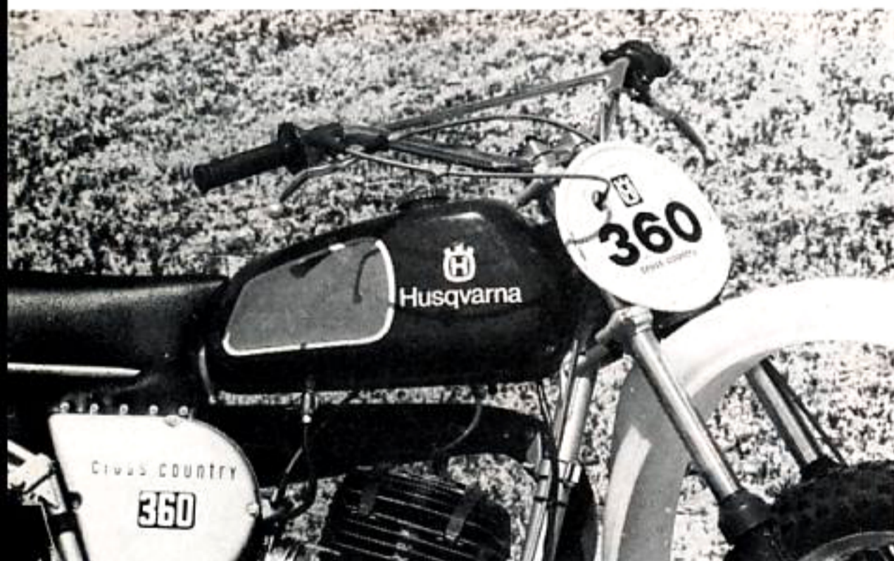
A big tank, Magura throttle, levers and grips, wide handlebars and a soft seat are all found on the WR.
