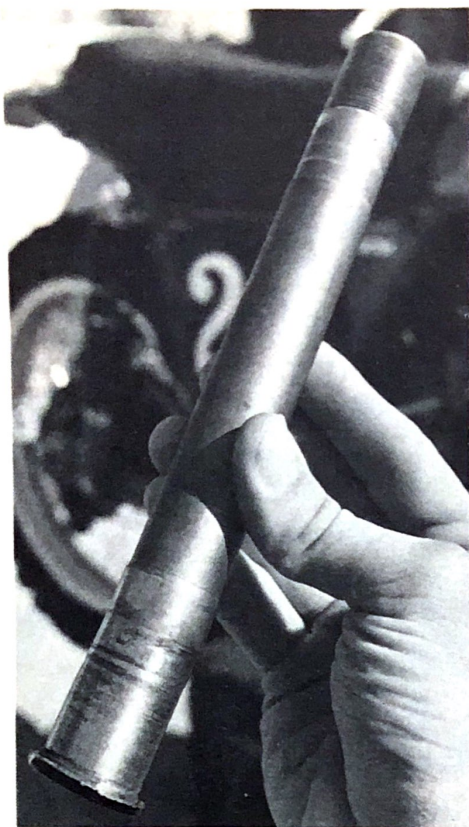
Honda steering stem bent like this after only two 15-minute motos. Made from low-grade Japanese moly steel.
