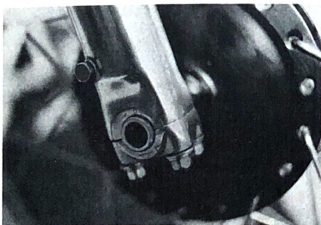
The Honda front axle bent after one race.
