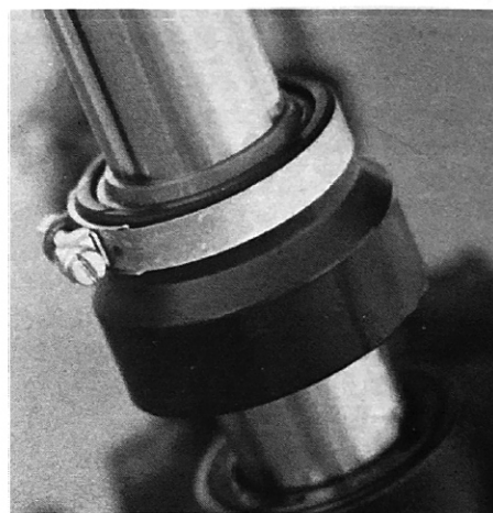
Nifty green plastic scrapers whisk away accumulated dirt before it gets to the seals. Our seals leaked after a short time, though probably not due to dirt.
