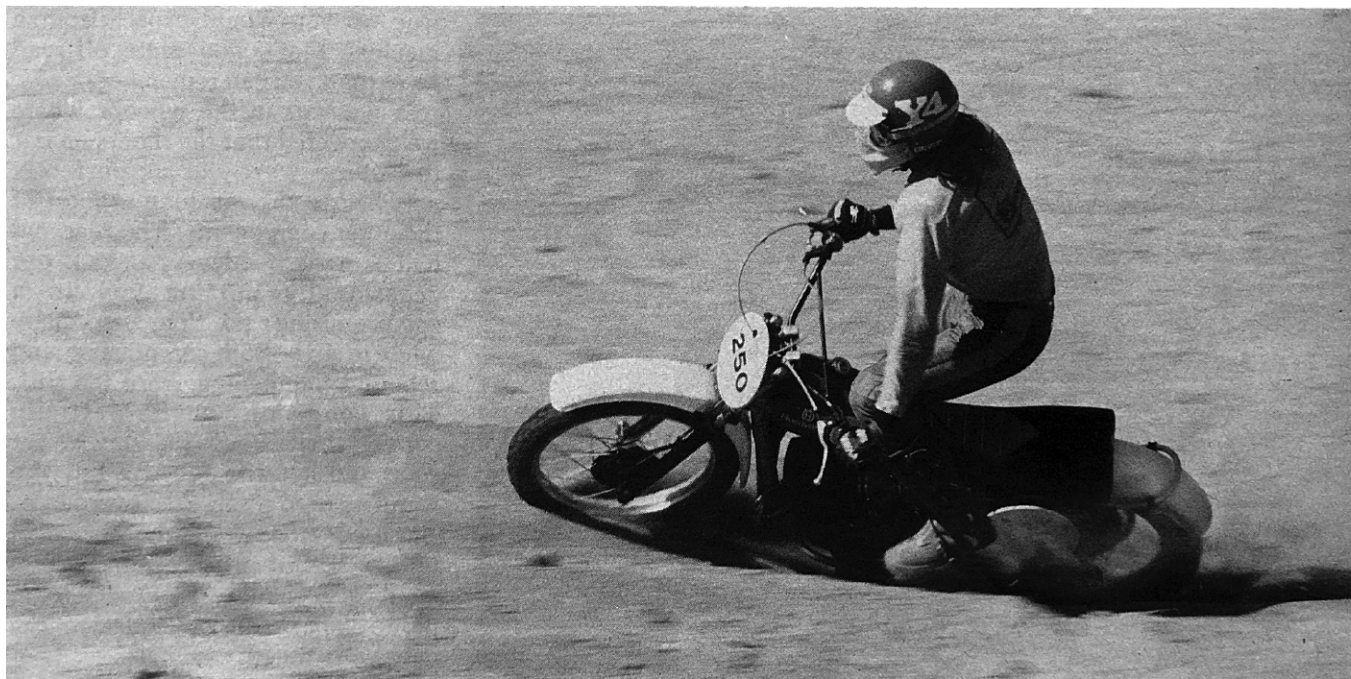
All but the final few millimeters of suspension travel, front and rear, are used in this deep sand turn.
