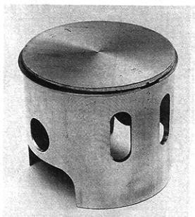
The flat-top piston is by Mahle. Slots mate with reed valve induction timing to charge crankcase.
