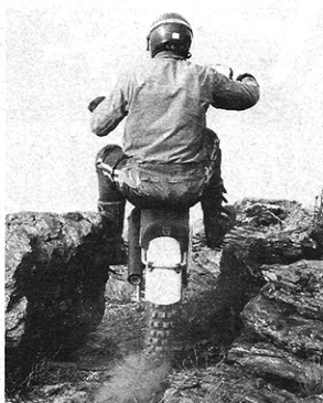
Barum 4.75 ISDT tire has a huge foot print and gives superb traction. Both rims are new-type Akront.
