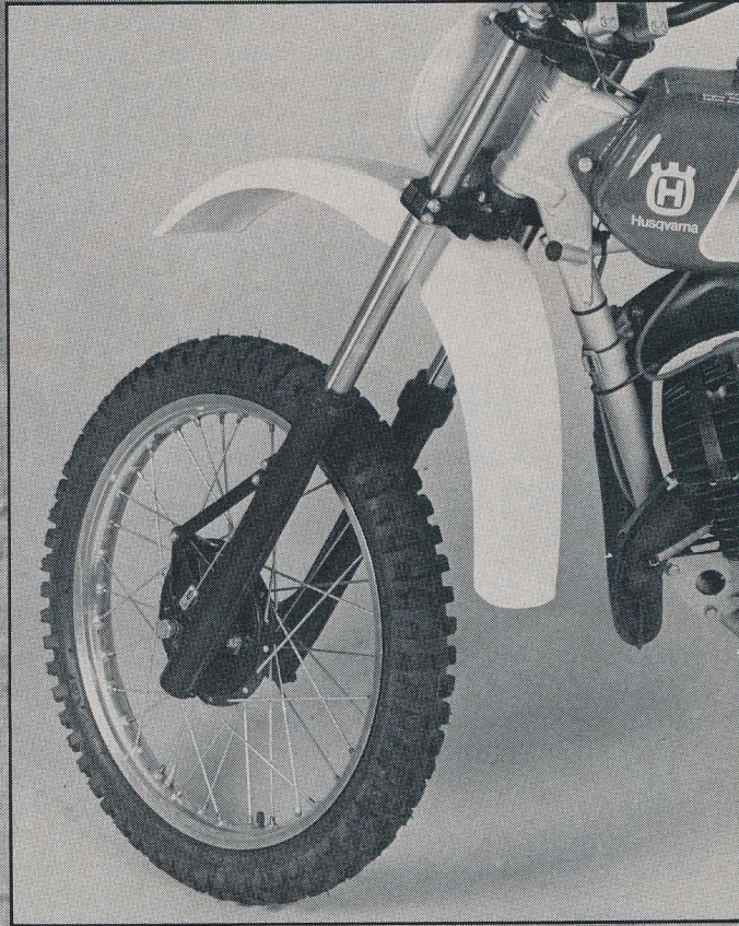
New 9.5-inch travel leading axle forks are bolted up to the newer MX-type conical hub and backing plate; it had the enduro-type full width hub last year.
