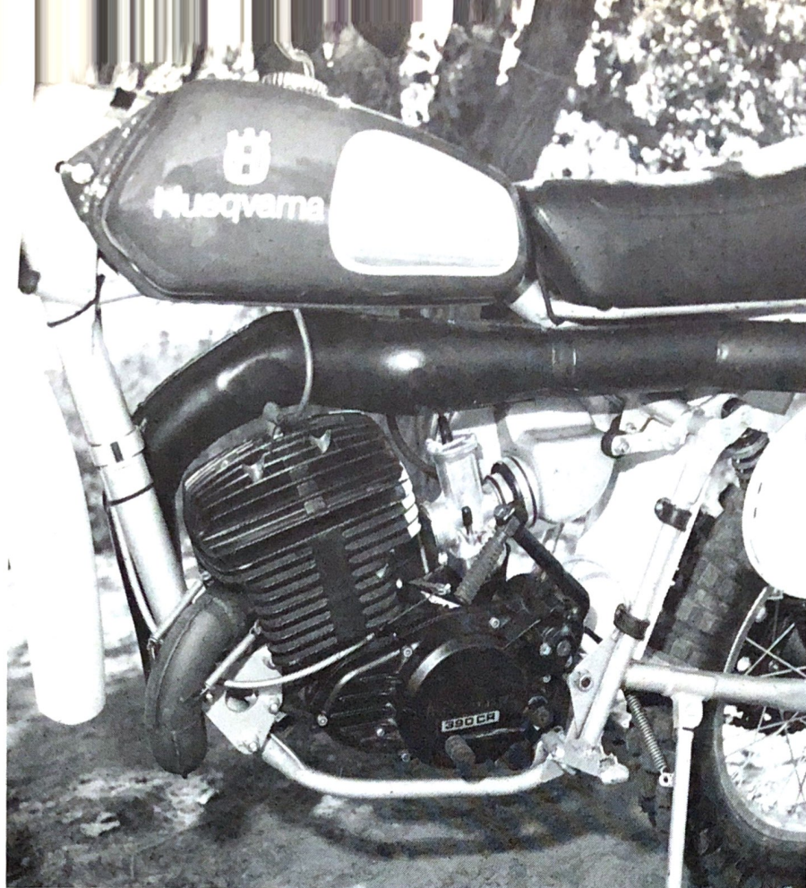
A 36mm Bing carburetor feeds the new 390 engine. Power changes are primarily from the longer stroke and new port design, which is identical to Brad Lackey's bike.
