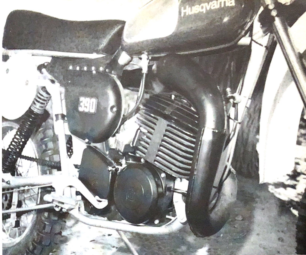
The snake pipe is well tucked in, but your leg still hits it up front if you scoot up up on the seat and keep your legs in tight on the tank.
