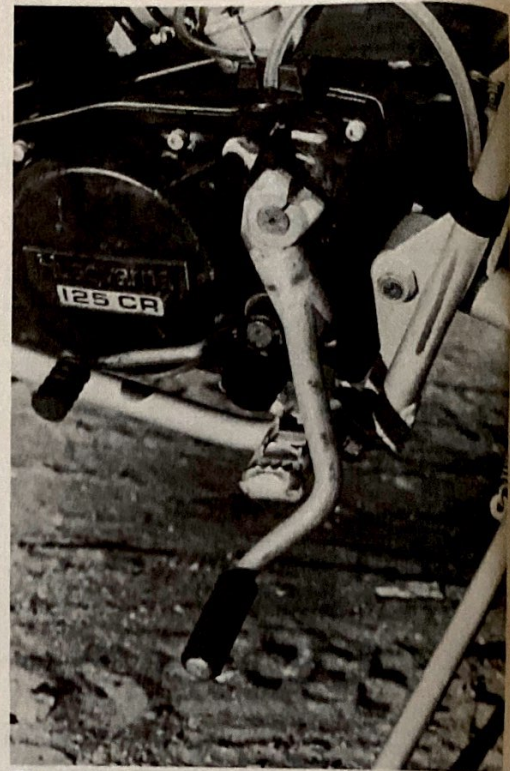
The kickstarter return spring snapped on the first day. It was the only failure during the test.
