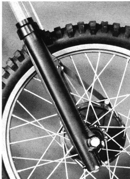
A standard oil/spring fork handles the front suspension. Accessory air-caps improve fork adjustability.
