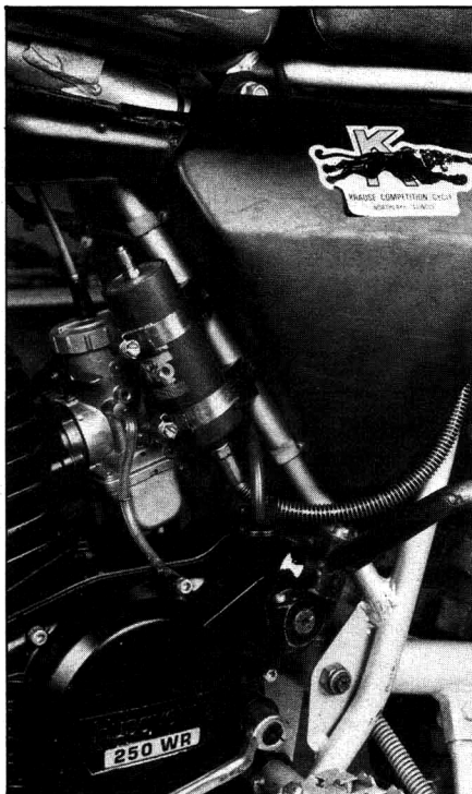
Left-side reservoir packs in tight to the carb. Pipe tucks in cleanly under side plate.
