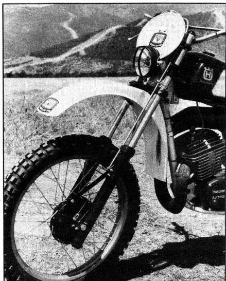
Forks are fine with zero air pressure. 3.50x21 tire is a little big for the stock fender.
