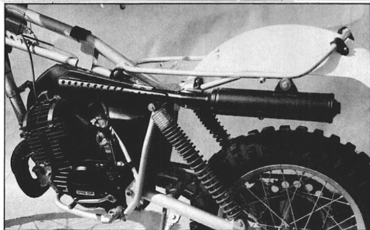
New pipe has a small heat shield on its rear cone. Engine has six-speed transmission with perfect ratios.
