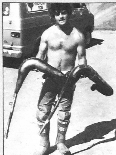
The greater volume and two-stage rear cone can be seen on the Asch pipe (left). The stock pipe doesn't do the job like the Asch model.
