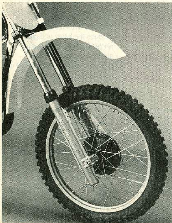
The new 40mm tubes and stanchions improve fork performance by reducing flex.
