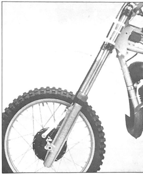
New forks have 40mm stanchion tubes and 11.8 in. travel.
