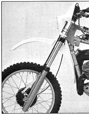
Both machines sport forks with 40mm stanchion tubes; the XC has 11.8 in. of travel, the WR 10.6 inches. Deep center aluminum rims are gold anodized for '82.
