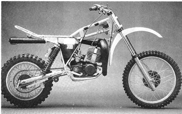
The off-road XC shares identical frame geometry, swing arms and suspension components with the CR 250 MXer.
