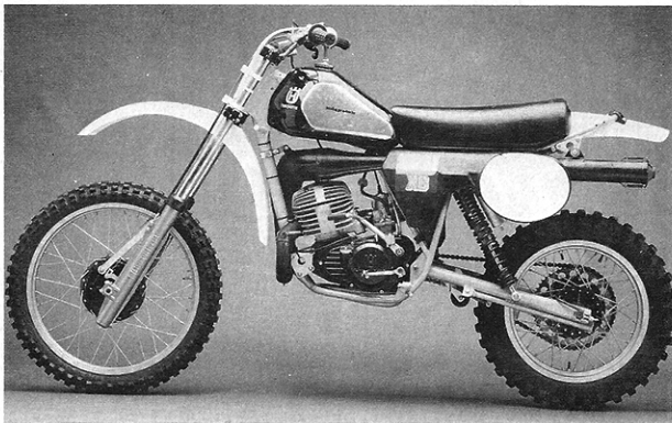
The XC employs a twin-shock rear suspension system that features excellent Ohlins piggyback dampers.
