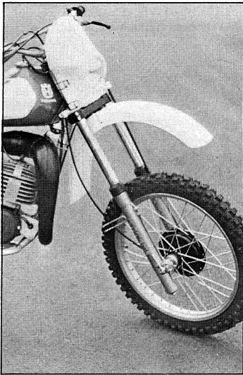
ABOVE Front 40 mm dia. motocross forks with travel shortened to 270mm. Wheel removal is considerably easier than your mate's CR (thank goodness).
