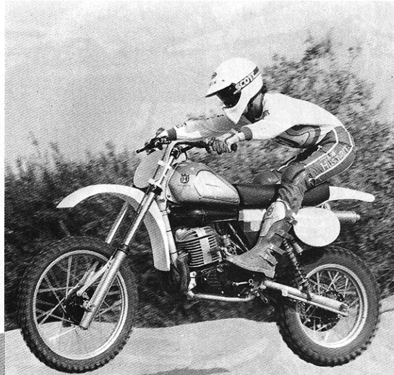
With nearly 12 inches of perfectly damped suspension travel, the big-bore Husky is a pleasure to ride anywhere.
