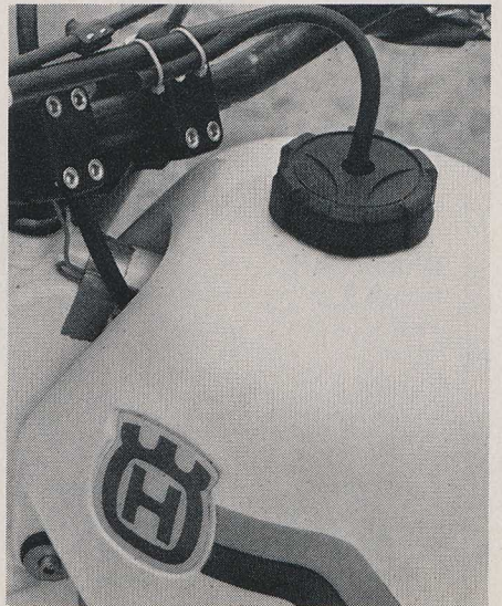
Another first for Husky is the white plastic gas tank (with reserve on the TE and TX).
