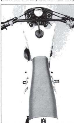
By not following the contours of the exhaust pipe very closely, the left-side numberplate makes the 400 excess uncomfortably wide just above the footpegs.
