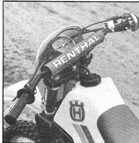
Up front it's all function. The seat fits nicely up the tank, while controls are excellent; only the combined lights/horn/kill switch needs relocating somewhere safer.
