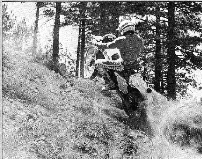
In tight woods you should drop the countershaft sprocket down a tooth. This will make the first three gears much more usable for tight terrain work. As it stands, the Husky sits a tad high for smaller riders, but it knifes through the trees with amazing accuracy.
