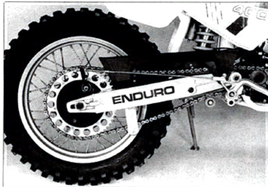
Improvements on the rear end include a lighter swingarm, a switch to a tongue-and-groove brake retention system and a new backing plate.
