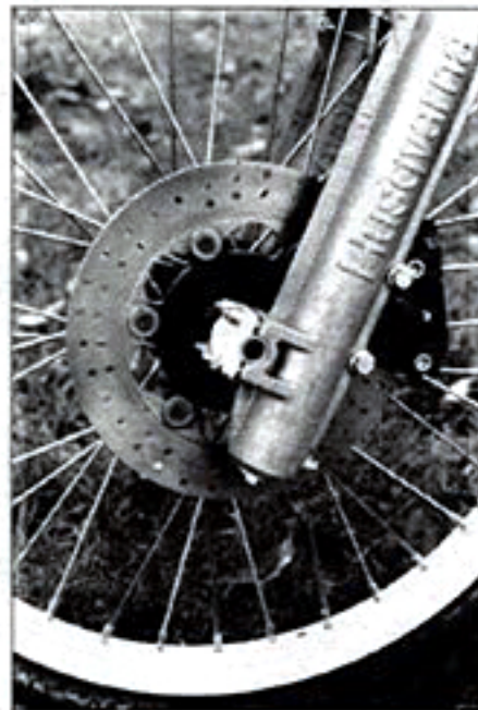
The 9.1-inch Grimeca disc is drilled and floats on its six mounts.
