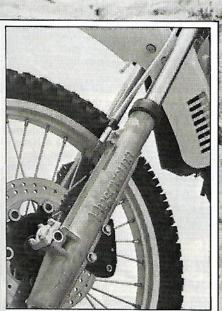
Marquis de Sade: These were good forks about four years ago, but the added power, height and demands of a racing four-stroke quickly turn these 40mm toothpicks into pieces of twisted, clanking metal.
