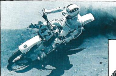
Ground swell: Water-cooling helped alleviate the Husky's overheating ills, but it also allowed the Swedish engineers to pump out more power. Good low end, steady mid-range and terrific top end can give the two-strokes fits.
