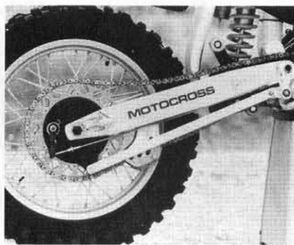
Although the full-floating brake setup performs adequately, a rear disc would certainly reduce unsprung weight and aid wet-weather stopping.
