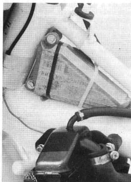
Husky's micro-processor ignition is similar to the KTM's except that it triggers the power valve, which kicks in at 6000 rpm.
