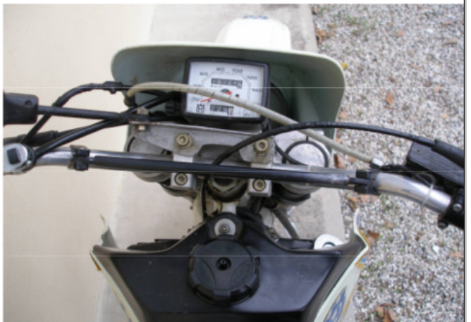
Frontlight mask is a mold of the "Cagiva Elefant" one. CEV Odometer. CEV Pushbuttons. Magura levers.
