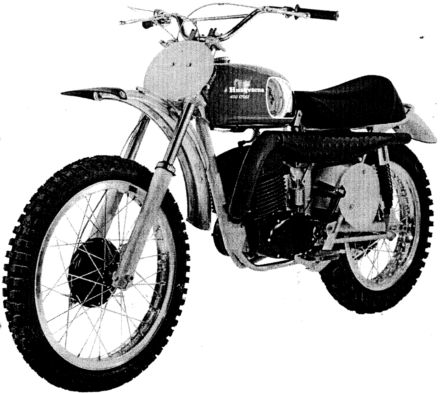
1970 Husqvarna 400 Cross, early model with 32 side float, steel tail, low decals, rigid pipe mounts, tab tank.
