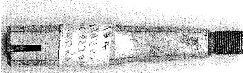
16 19 653-01 MotoPlat stub - 125 motors 72 thru 87 - actual size Same taper fit as 16 10 851-01 shown above
