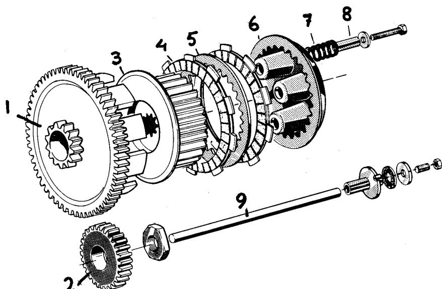
1. 16 11 669-01 Kopplingskrans, clutch gear
